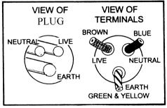
Wiring Arrangement of connector-cable
