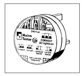
Even when the site connector is to EN60309-2, UK caravanners can still encounter the problem known as *reversed polarity*. This is where the site supply's 'live' line connects to the caravans 'neutral' and vice versa and is due to different standards of plug and socket wiring that exist in other countries. We therefore recommend checking the polarity immediately on connection, using a polarity tester. One tester available from most caravan accessory shops is made by W4.
