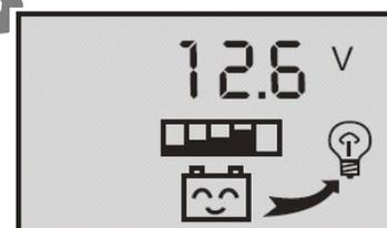
At this interface, press button
