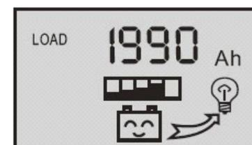
At this interface, press button
