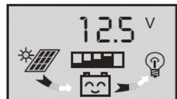
This interface is the main interface, and it shows the charging & discharging state, battery capacity and battery voltage.
