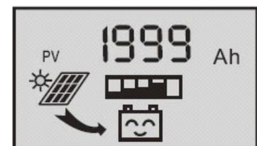
At this interface, press button
