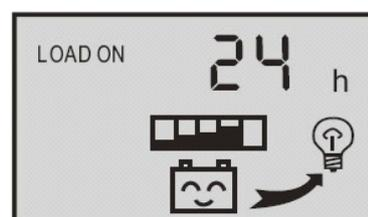
24h — indicating normal mode, loads are under the condition of supplying power without breakdown;
