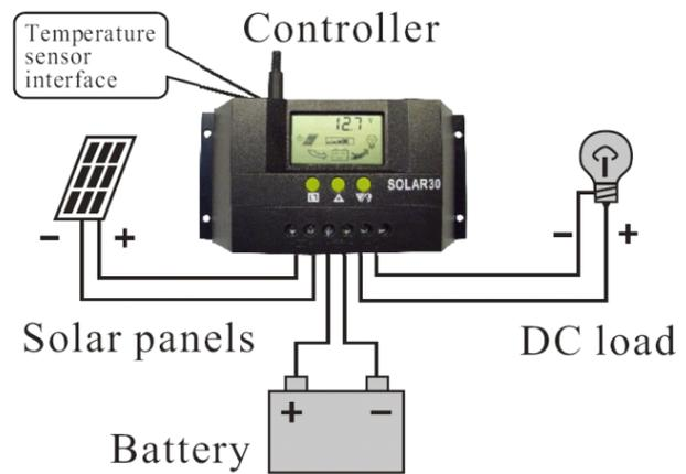
**Disassemble:** To avoid the accident, please dismantle the solar panels, battery, loads from the controller in order.
